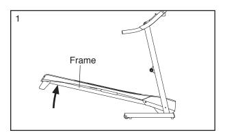
Hold the treadmill firmly with your right hand as shown. Pull the latch knob to the left and hold it.
